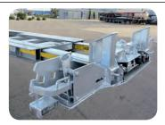
**Option 1:** front extension for 45' container loading within legal maximum length (without special transport permits)
