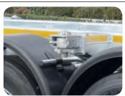
**Option 2:** extra twist locks in front part for advanced 20' container, to increase adherence in traction motor.
